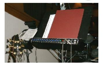
Photo showing a MyMix14 headphone monitor box mounted to the bottom of a tall music stand keeping the controls within easy reach whether standing or sitting while playing.
