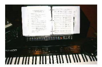
Photo showing a MyMix14 headphone monitor box mounted to the bottom of a music stand keeping the controls within easy reach for the electronic keyboard player to adjust the mix or mute the keyboard while setting up a blended patch of several MIDI modules thus hearing the sounds in the headphones but being muted in the house AND in all other monitor mixes including all MyMix14 boxes.
