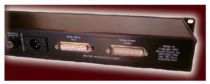
On the right rear panel are two multi-pin connectors that brings the audio and external power supply into the MyMix14. You can keep adding MyMix14 units with the addition of our twisted-pair master cables. These cables are available in lengths 6', 10', 15' 20', 25' and 50'. A standard MyMix power supply can handle up to 10 MyMix14 units. An larger power supply is available for larger installations.
