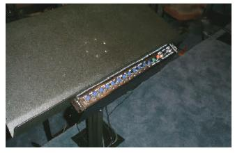
Photo showing a MyMix14 monitor box mounted to the bottom of a extra wide directors' music stand allowing the director to make changes to the monitor mix even while directing an orchestra or choir.
