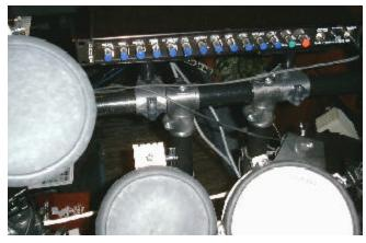
Photo showing a MyMix14 headphone monitor box mounted to the drum rack directly in front of the drummer again keeping the controls within easy reach to adjust the mix. Drummers like the low-end that acoutic drums provide. These electronic drums feature a "Subwoofer Shaker" mounted to the drum throne letting the drummer "feel" the low end thru the seat but not putting those low frequencies out into the house.
