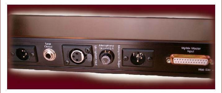
In the center of the rear panel is a microphone input and an microphone "feed thru" to pass the microphone level signal on into the house system. A ground lift switch is also provided for this microphone tap.
